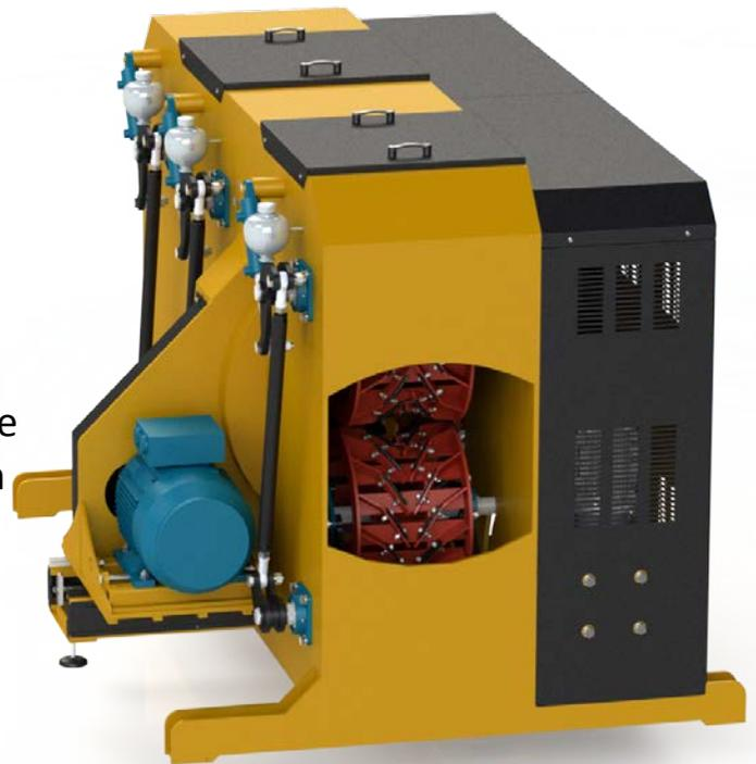
The rotor uses a high-quality ball slewing bearing with a polymer separator that does not require constant lubrication, but only periodic service. The machine case **SKYWOOD DB-600** has a welded frame made of thick sheet metal, which is quite heavy, which reduces the level of vibration and noise of the machine.
