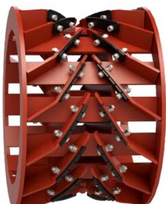
For reliable long-term operation of the pressure rollers, the hardox wear-resistant steel plates are installed on each of them. If worn out, the plates can be replaced with new ones.
